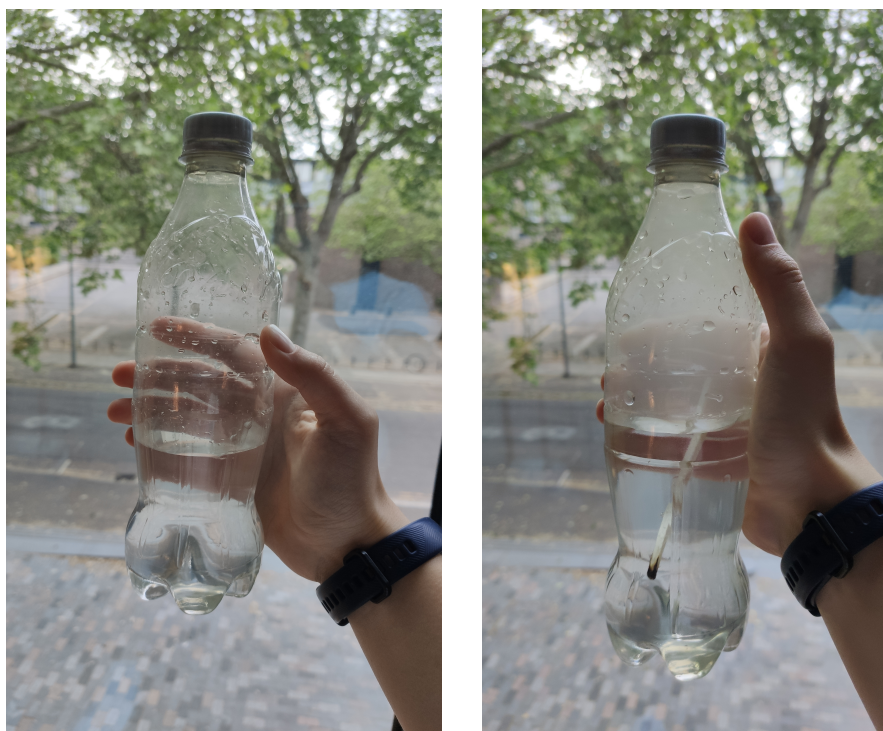
Figure 1: Results of the experiment: nothing happens in the bottle before adding the match (left); the air in the bottle becomes cloudy upon squeezing and releasing after the match has been dropped (right).
