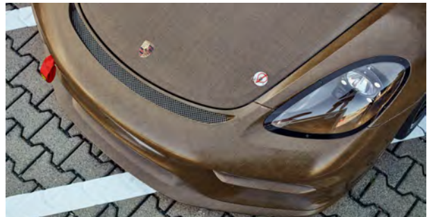
Figure 2 - Porsche bodywork made from natural fibres
