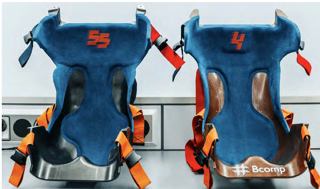
Figure 3 - McLaren F1 seat, carbon fibre (left) and flax fibre (right)
