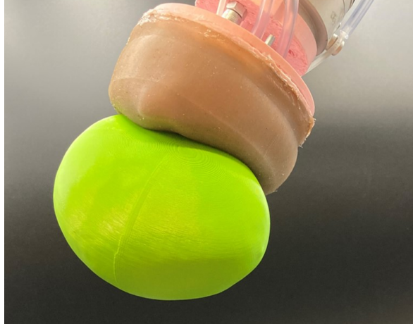
Figure 1: Novel Soft Gripper holding a 3D printed Mango (in Green)
