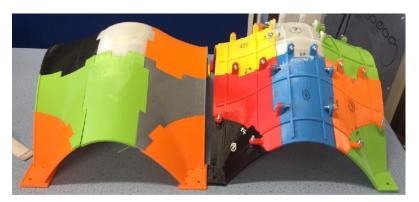
3D printed mould used to cast model shells of the Droneport
