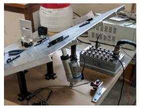
The designed tilting table with connected apparatus including the driving actuator
