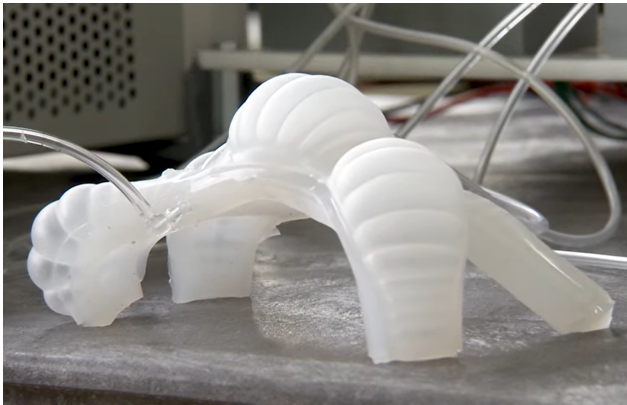
(a) Soft, pneumatically-actuated crawling robot invented by NASA [1].
