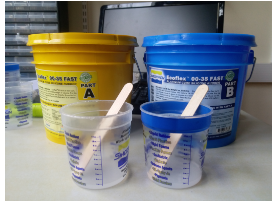
(b) Raw material silicone consists of two components, named part A and part B.
