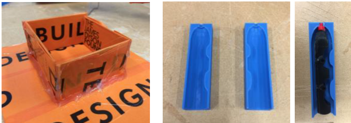
(a) Simple mould made of cardboard. (b) Mould for fabricating soft prosthetic finger.
