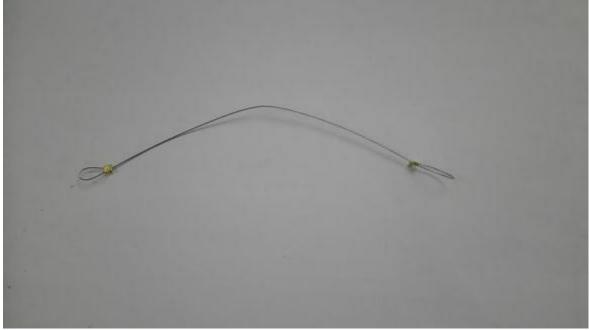
Figure 2: On of the wires which was threaded through the biscuits for testing. The mass hanger was suspended from the loops at either end.
