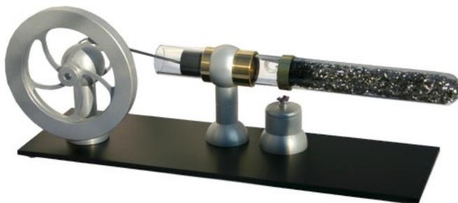
A purposely-made thermoacoustic piston engine
