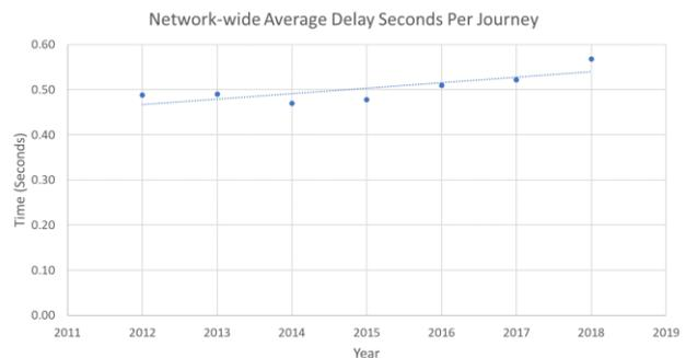
FIGURE 2: DELAYS SCALED BY NUMBER OF JOURNEYS THROUGH TIME.
