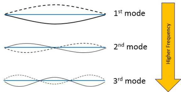
FIGURE 9: MODES OF PINNED STRING VIBRATION.
