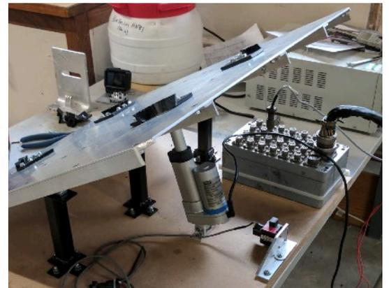
*The designed tilting table with connected apparatus including the driving actuator*
