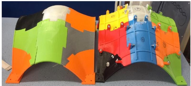
*3D printed mould used to cast model shells of the Droneport*
