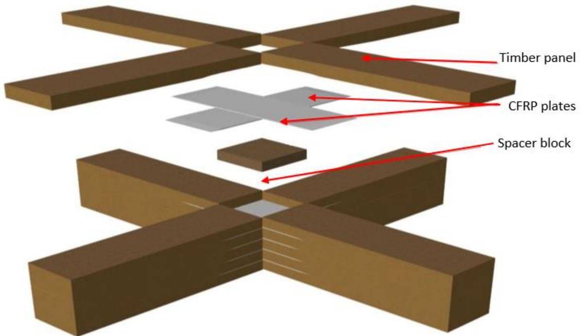
*Figure 3: Idea for the diagrid connection with multiple CFRP plates*
