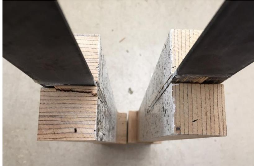
*Figure 5: Image showing parallel (left) and perpendicular (right) orientation*
