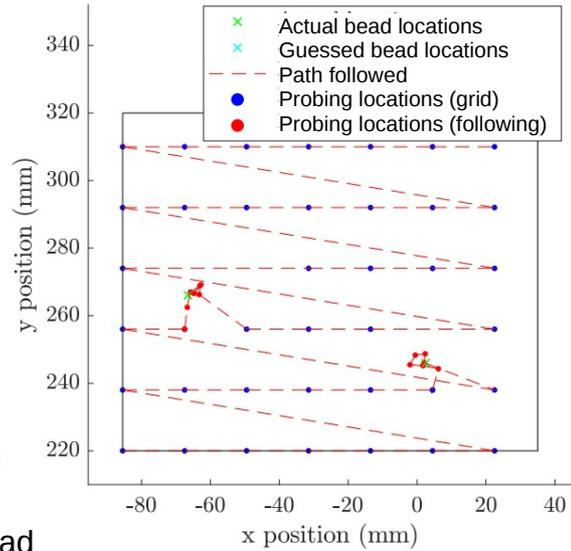
Locations where the robot had to probe during this test
