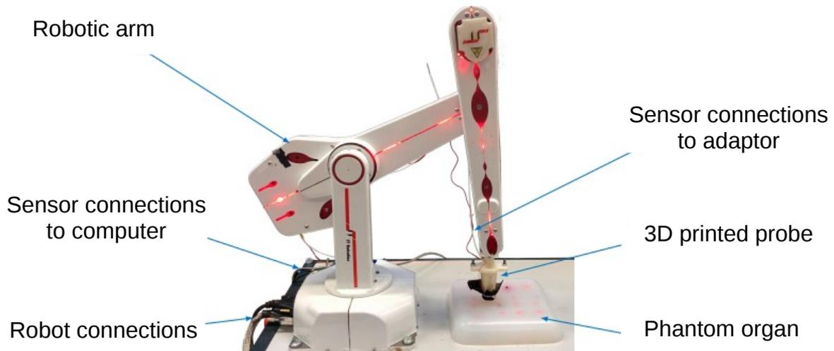
The robot was programmed to perform two separate tasks. The first was to try and find the beads within the phantom organ. The probe was pressed vertically downwards to a fixed depth and a tactile image recorded at this point. The task was to decide where to press down next, given the previous information, to reduce the total number of locations the robot had to probe.
