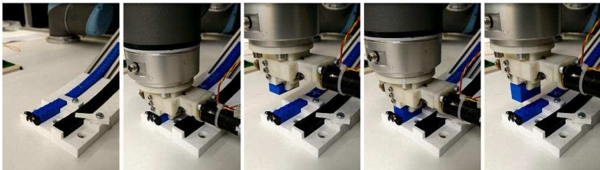
The feed system can provide up to 2 types of bricks to the robot. The robot can store bricks in the feed system and even use it for simple prefabrication.
