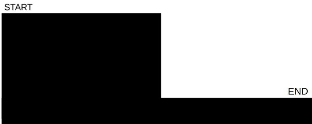
So the motor needs to turn left when the sensor is on black, and turn right when on white. We can use the difference between the light sensor measurement now and the measurement on black or white to control the motor power.
