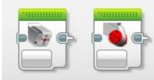
Add one of these blocks after the “stop motors” block to close the gripper and pick up the ball!
