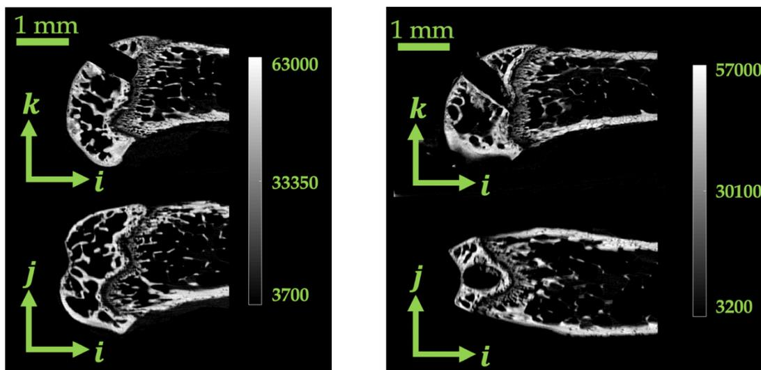
Figure 3 - CT scans of drilled hole (left) and needle hole (right)
