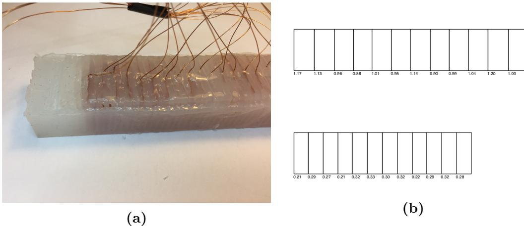
**Figure 3:** (a) The axial prototype (b) Representation of the visualization of deformations in the axial prototype.
