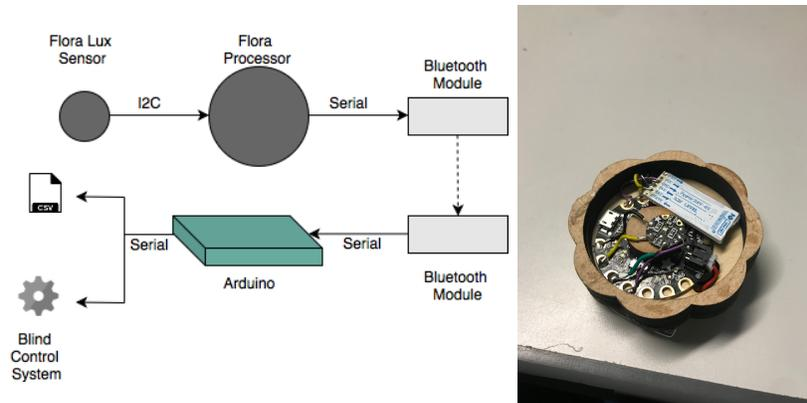
Figure 2: Wearable Light Sensor Developed As Part Of The Project
