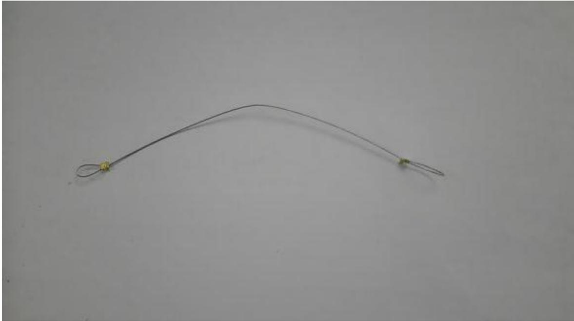
Figure 2: One of the wires which was threaded through the biscuits for testing. The mass hanger was suspended from the loops at either end.
