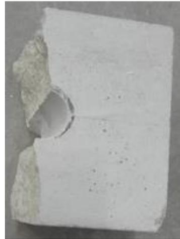
^Figure 4: Comparison between model and test sample for 50 mm edge distance
