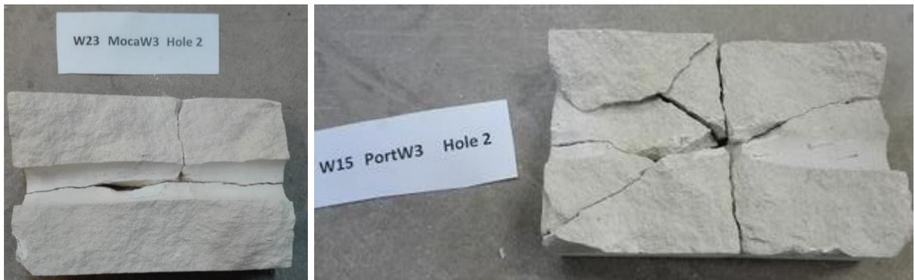
^ Figure 5: The two types of failure observed when edge distance was 25 mm
