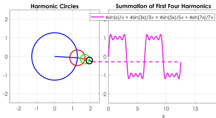
Figure 2: Addition of harmonic tones to produce an approximate square wave.
