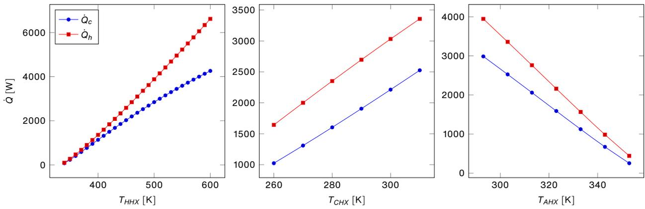
Power flux variation with heat exchanger temperatures
