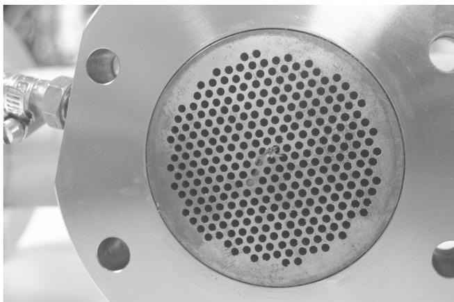
Proposed heat tube-shell heat exchangers
