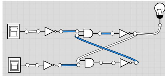
An extension was planned to fill any remaining time in case the students were very proficient at the other activities. They were shown the circuit above and asked to work out what it does. This would have been used to explain how feedback could be used to “remember” previous states, and how bistable circuits can form the basis for primitive memory cells and state machines.
