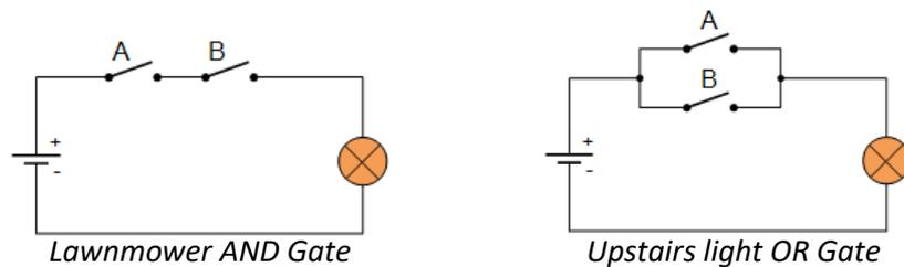
The students were then challenged to combine the three components into circuits which would perform specific functions. These were designed in pairs/groups of three. The problem statements were:
