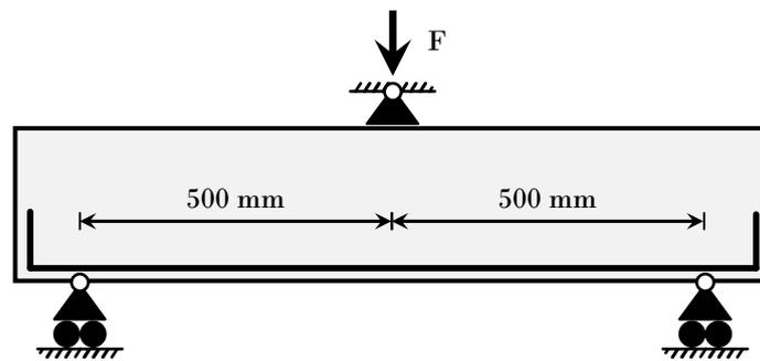
Figure 3: Three-point bending
