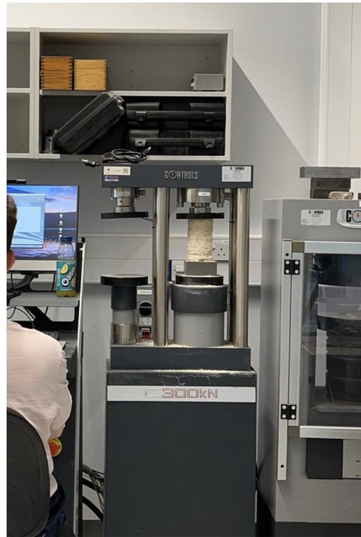
Figure 5: Compression tests of core samples
