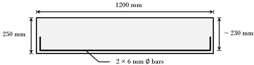
Figure 2: Dimensions and reinforcement layout of rammed earth beams
