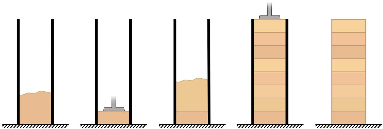
Figure 1: The construction of a rammed earth wall
