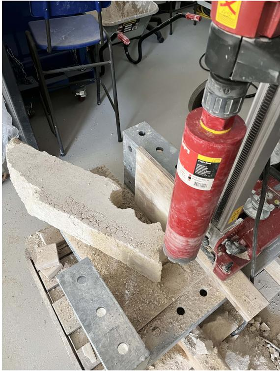
Figure 4: Core drilling machine
