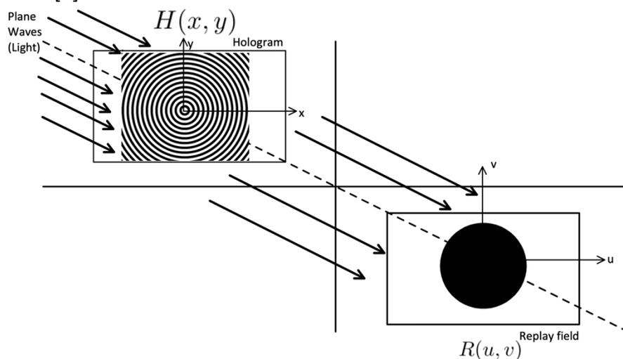
Figure 1 - Diagram illustrating holography
