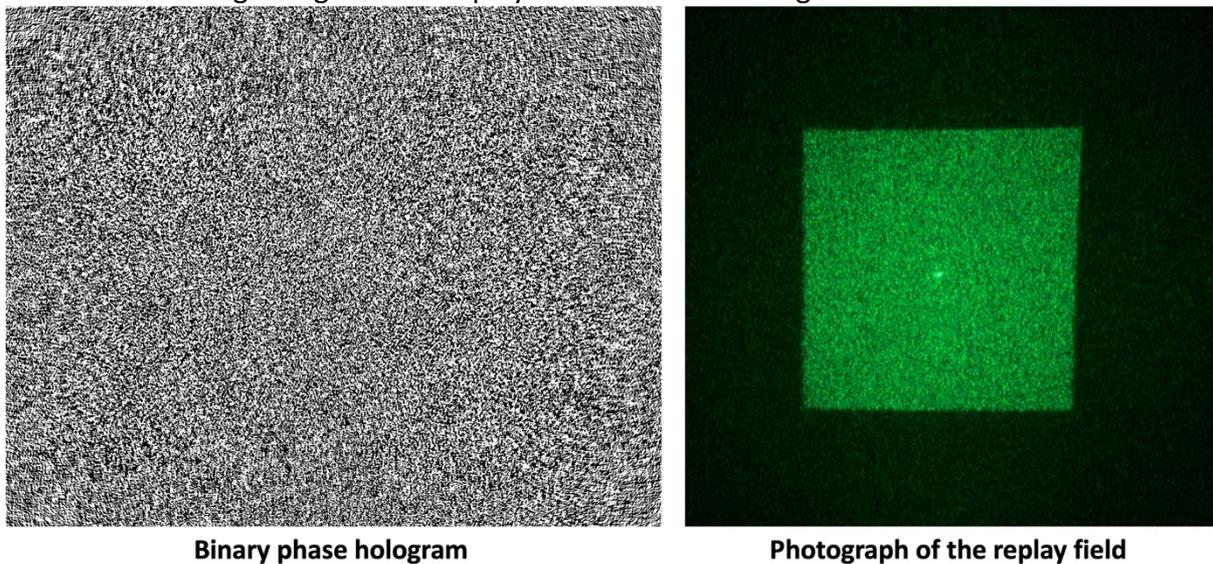
*Figure 5 - Hologram and replay field displaying a square generated by the new method*
