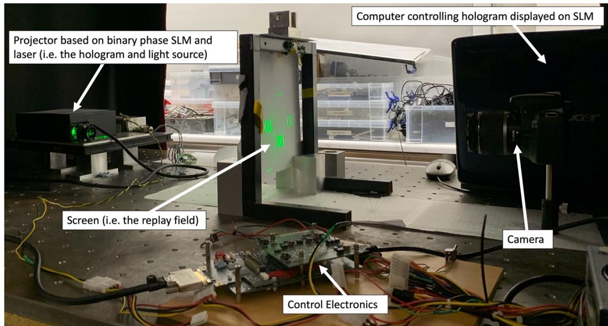
Figure 2 - Experimental setup of holographic projector
