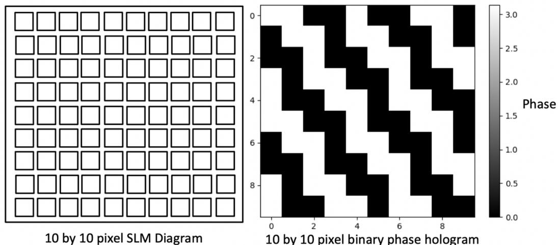
Figure 3 - Diagram showing a binary phase spatial light modulator (BP-SLM)
