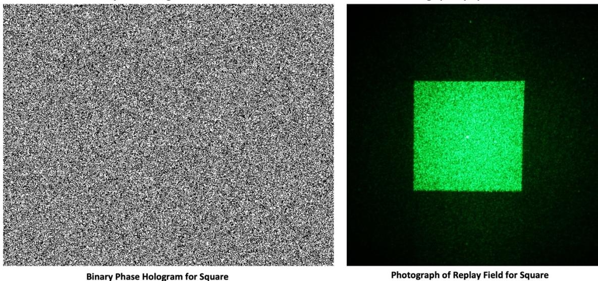
Figure 4 - Hologram and replay field showing a square generated by the Gerchberg-Saxton algorithm
