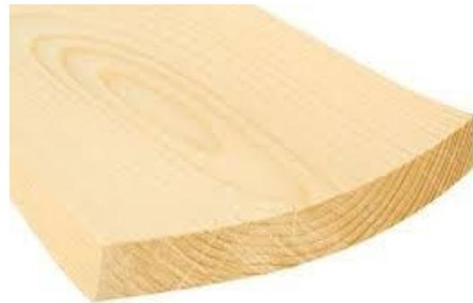
Figure 3 - This wood has warped
