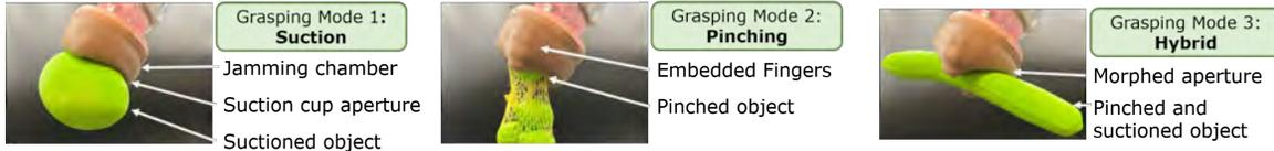
Figure 1: Different Modes of Novel Soft Gripper
