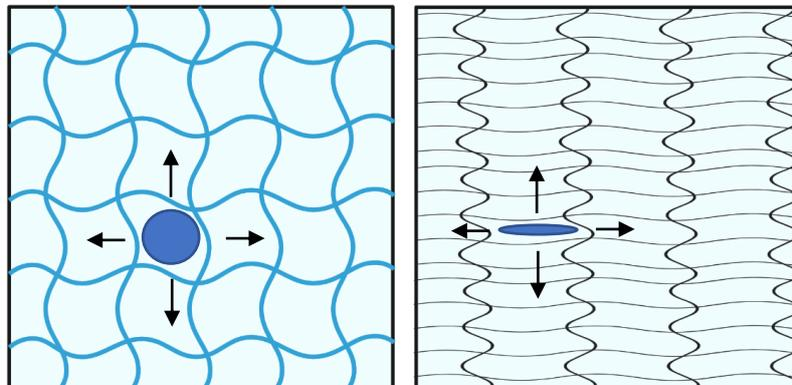
Figure 5. Crystal growth in an isotropic (left) and anisotropic (right) hydrogel structure.
