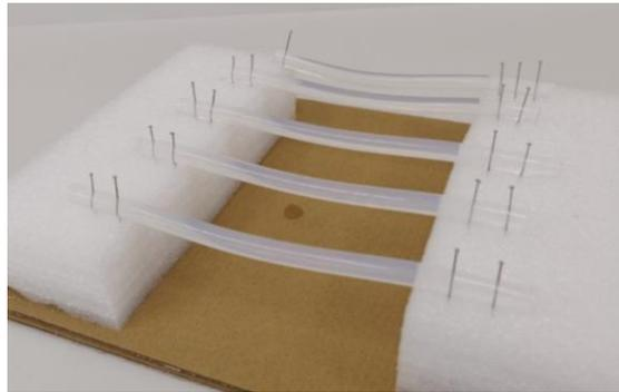
Figure 4. Drying hydrogel fibres under tension.
