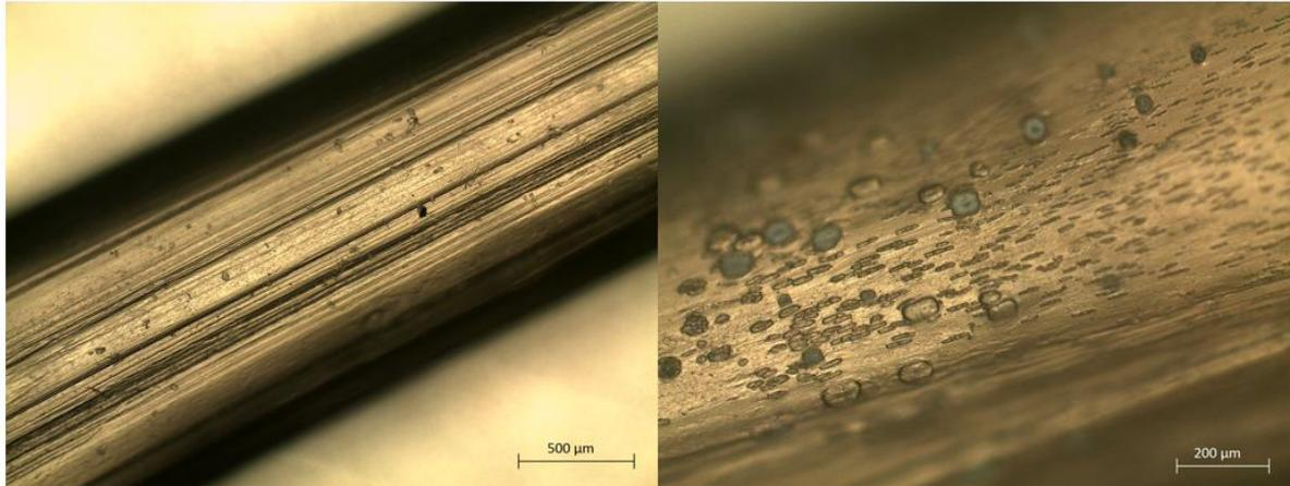
Figure 6. Light microscope images of crystal precipitation in dried anisotropic hydrogel fibres.
