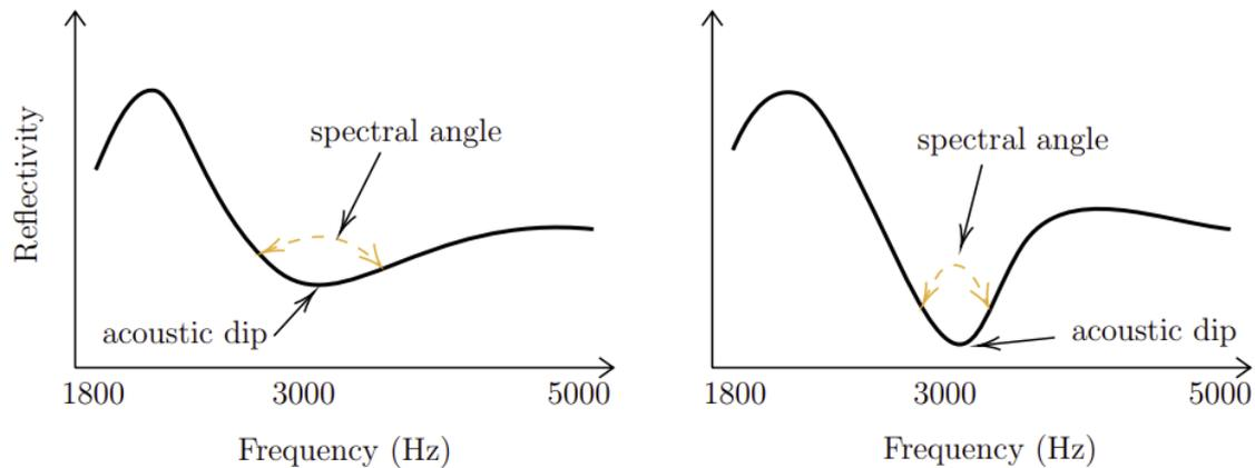
Figure 1: Plots of the output from acoustic reflectometry of a healthy ear (left) and an effused ear (right). The spectral angle is labelled and is narrower for the effused ear.
