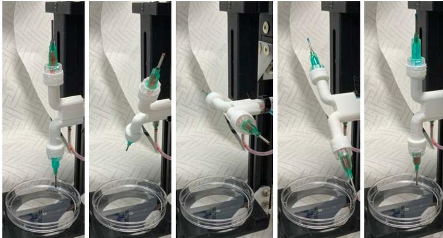
Figure 4: Automated Printhead Switching
