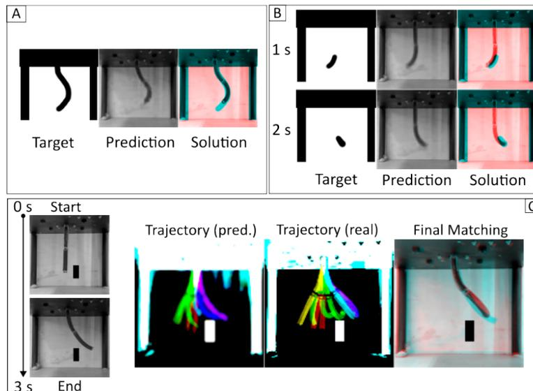
Figure 4: (A) Robot control with a hand-drawn shape target (B) Robot control with only the tip drawn as a target (C) Obstacle avoidance: attempting to achieve a robot shape without colliding with the box
