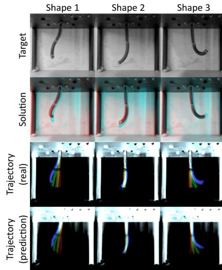
Figure 3: Three different targets that the robot must achieve in 3 seconds. The solutions (red) are shown mixed with the target (cyan) for comparison. The trajectories follow the movement from red to violet
