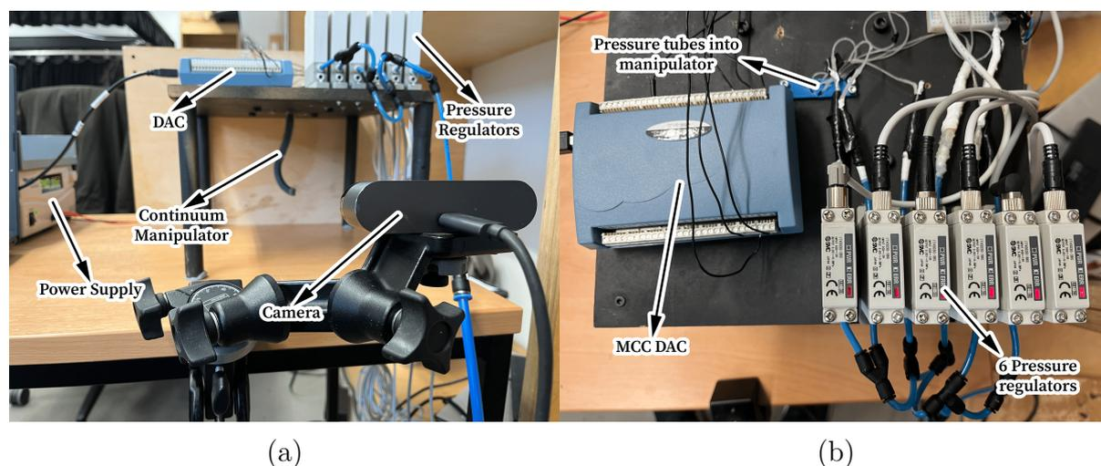
Figure 2: (a) A fixed camera records the robot’s movement (b) Voltage signals sent through a circuit control the pressure to 6 tubes built into the robot
