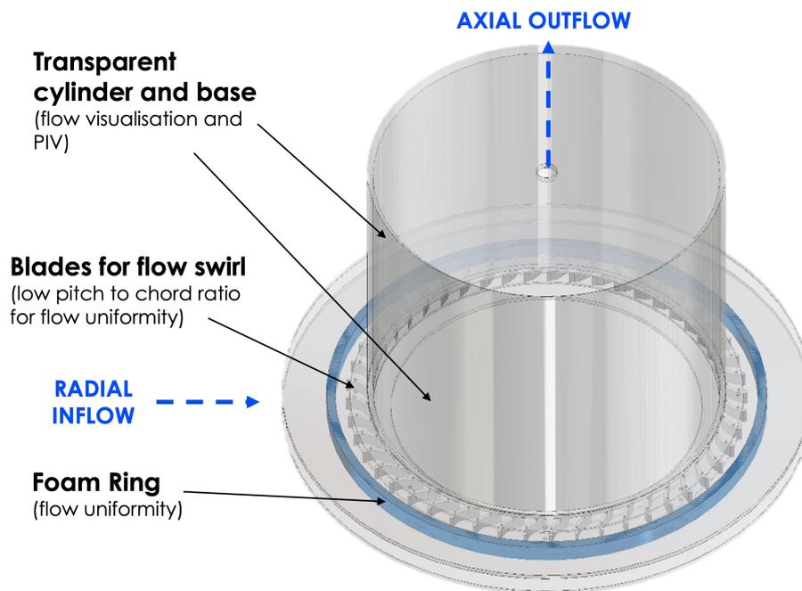
Figure 4: CAD model of the experimental apparatus
