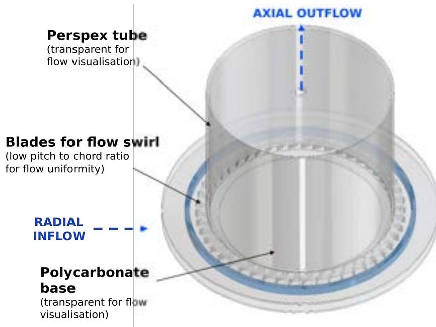
Figure 2: 3D CAD model of the vortex chamber
