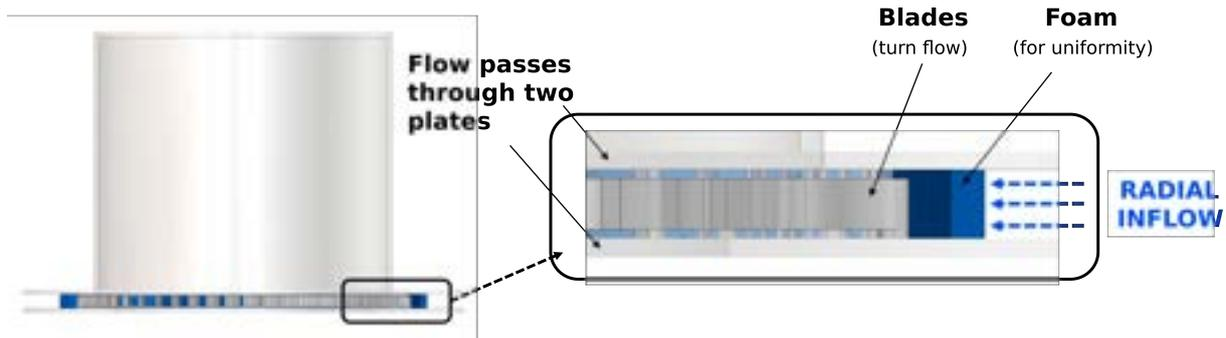
Figure 3: Flow path at entry to the chamber
