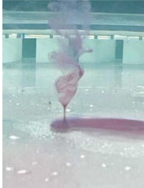
(b) Axisymmetric bubble breakdown
