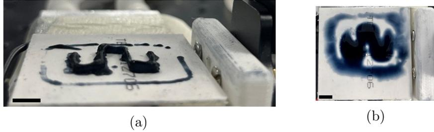
**Figure 8:** (a) Cryoprinted 5-layer square wave structure before thawing. (b) Cryoprinted 5-layer square wave structure after thawing. All scale bars represent 5 mm.
