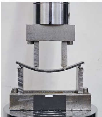
Figure 8: 4-point bend test rig showing the 2.7mm CFRP sample
