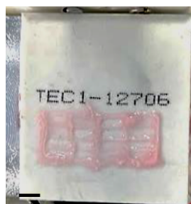
Figure 3: Cryoprinted alginate-hydrogel grid, crosslinked with calcium chloride and thawed.
