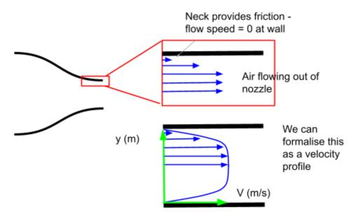
We can see that there's a flat section to the velocity profile in the middle referred to as the freestream and near the walls there's thin layers where the velocity rises from zero to the central velocity. These are called boundary layers. (Similar concept as the tornado boundary layer but much simpler).
