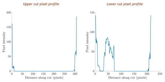
Figure 5 - Pixel intensity profiles along upper and lower cuts of hole
