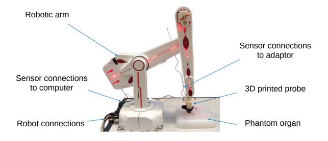
The robot was programmed to perform two seperate tasks. The first was to try and find the beads within the phantom organ. The probe was pressed vertically downwards to a fixed depth and a tactile image recorded at this point. The task was to decide where to press down next, given the previous information, to reduce the total number of locations the robot had to probe.
