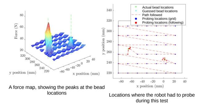
The other task was to look into how the robot could determine other things about the beads, such as their size and depth, once they'd been found. This is similar to how a doctor could tell how dangerous a tumour is by feeling how large it is. We looked at how far you need to press straight down on a bead to accurately decide this, and also whether it's better to rotate the probe as well.
