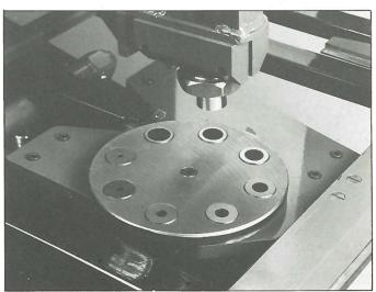
Where regular punching of different size holes up to 18mm dia is carried out, a special Bolster and Turret assembly is available, which enables rapid changeover from one hole size to another.
