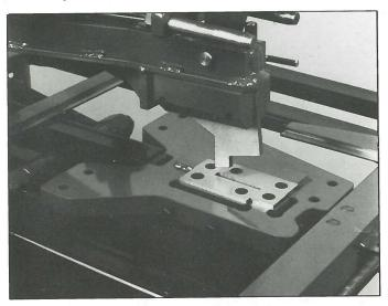
Each machine is fitted as standard with a 50 x 6mm heeled blade and 4 piece adjustable die on type 'A' Bolster. One stroke cuts a slot 50 x 6mm in up to 3.2mm thick mild steel. Longer slots are cut by successive strokes and shorter ones by using the Stop Screws as illustrated on page 5. Shorter and thinner blades are also available.
