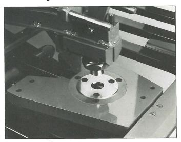
Type 'B' Bolster is available together with a range of circular punches and dies for holes from 2 to 75mm dia. Punches and dies align automatically after initial setting of the Bolster. Special tools can be supplied for larger diameter holes.
