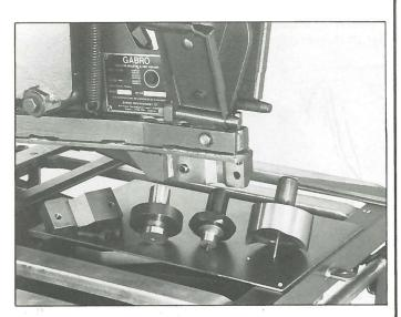
With the blade removed, the top tool clamping block has two split bores which permit exact positioning of punch holders of either 1" or 25mm dia. Square ground punches are set at 2° to provide "shear". For extra punching capacity "claw shear" punches are available.
