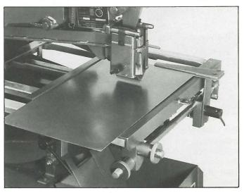
Side and Rear Fences are fitted to all machines as standard, each with a quick release for rough positioning. Fine adjustment is provided by a knurled handwheel and once set up the fences can be locked in position by a tommy nut clamp. An Extended Side Fence is available for use with larger sheets of material.
