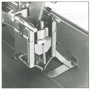
A Line Guide is also fitted, for use when fences are impractical. The nib, seen here just touching the line, is arranged to indicate the exact position of both the sides and front end of the die, usually hidden by the workpiece. When not in use it can be swung away and is relocated by an accurate ball plunger.
