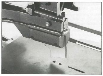
Two knurled Stop Screws control the depth of entry of blades and punches into the dies. The block on which the longer screw abuts is pivoted so that it can be swung in or out of use instantly. The setting illustrated is typical for making a small slot where only the top of the blade is required to enter the work, which is then turned and the slot completed from the other end.
