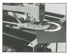
Circumferences finish as a series of short flats and this is generally acceptable without further work, as the out-of-round, using a 25 x 6mm blade, is only 0.5mm at 300mm dia. This is a quick way to cut out large holes and discs to about 800mm dia and in up to 3.2mm mild steel. Radial slots are also simple to achieve.
