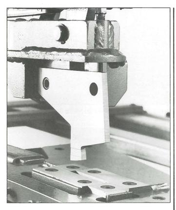
The blade pivots on a bush with adjustment at the front provided by a vertical screw. This arrangement gives fine adjustment for correct clearance between the back of the blade and the die, whilst correct clearance at the front of the blade is controlled by adjustment of the die itself.
