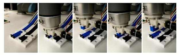
The feed system can provide up to 2 types of bricks to the robot. The robot can store bricks in the feed system and even use it for simple prefabrication.
