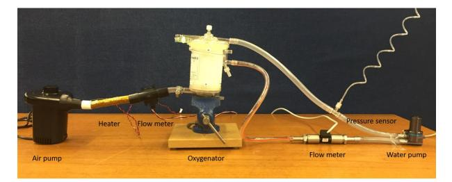
Once the system was all set up, as seen above, with all the sensors and control working, I was then able to investigate whether using air would actually heat the blood up to a sufficient temperature. Many tests were run to determine this. One example is to look at
