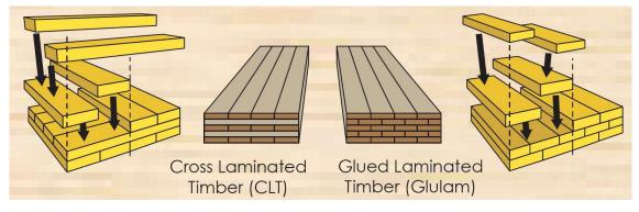
Figure 1: CLT vs glulam, two engineered timber products.
