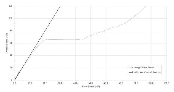
Figure 8: Average of the force in each of the four plates versus overall force for test A4
