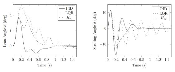
Figure 3: Simulated Bicycle Controller Response
