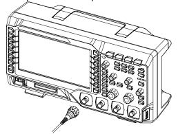
Figure 5 To Connect the Passive Probe
