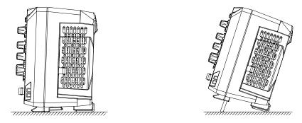
Figure 3 To Adjust the Supporting Legs
