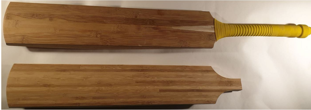
Figure 3: Face of prototype bamboo cricket bat and blade produced by Garrard & Flack.
