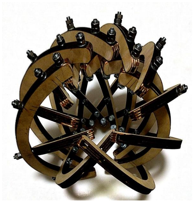
CAD model of the framework designed for planar deployable sliceforms for experimental testing, and an assembled prototype wooden sliceform using offset members
