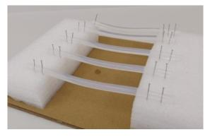
Figure 4. Drying hydrogel fibres under tension.
