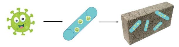
Figure 2. Hydrogel fibre-encapsulated, bacteria-based self-healing concrete concept: Bacteria are first encapsulated in hydrogel fibres and then distributed throughout a concrete matrix along with a food source for the bacteria.
