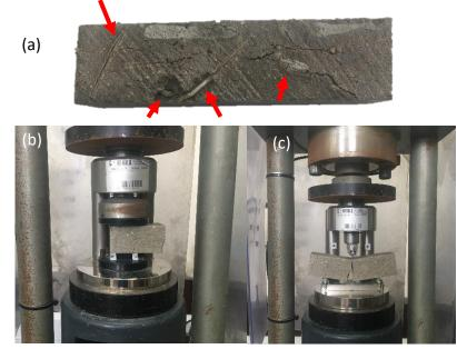
Figure 7. Mortar specimen making and testing: (a) Hydrogel fibres are mixed into the mortar to make fibre-reinforced specimens, (b) Testing under compression, (c) Testing under flexion.
