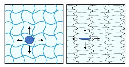
*Figure 5. Crystal growth in an isotropic (left) and anisotropic (right) hydrogel structure.*
