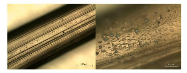
Figure 6. Light microscope images of crystal precipitation in dried anisotropic hydrogel fibres.
